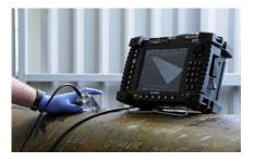
A PAUT is more robust and easier to use than conventional single-element probes, providing improved efficiency, capturing hundreds of signals at once, and reducing the number of false alarms. PAUT provides a permanent record. And because PAUT can detect defects at the surface and into the volume of a weld (with no dead zone), it also gives information about the lateral position of a defect (depth and height).
